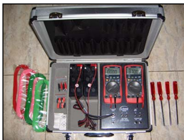
Gambar 1. Alat resistivitas G-Sound
