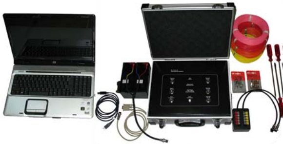
Gambar 1. Alat resistivitas S-Field 16 elektroda otomatis multichannel
